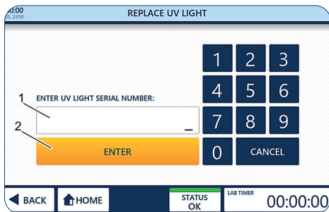
Fig. 24: Activate the automatic life time surveillance for UV light
