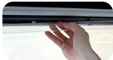
Fig. 51: Rotate the UV lamp
