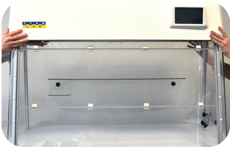
Fig. 12: Lift the top housing onto the PC glass chamber
