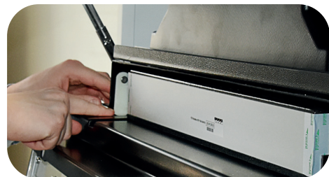
Fig. 48: Lift the HEPA filter housing up
