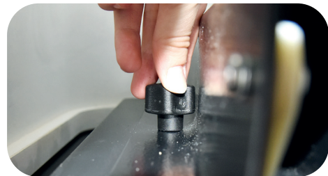
Fig. 47: Open the screws by two or three turns
