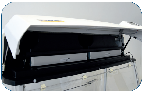
Abb. 53: Opening the lid of the upper housing part
