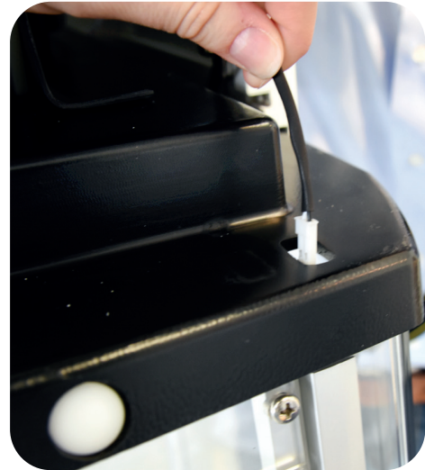
Fig. 16: Connecting the magnetic safety switch
