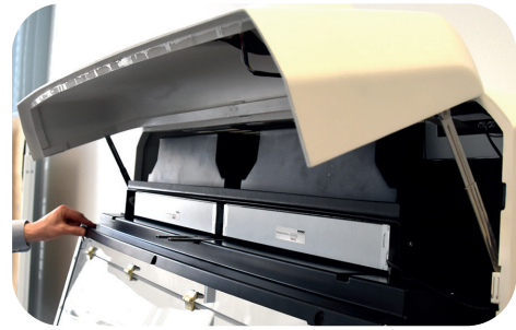
Fig. 15: Fix the front side of the top housing
