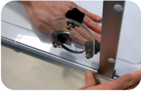
Fig. 7: Fix the right side panel to the base plate
