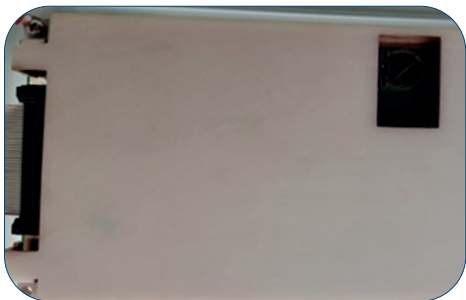
Abb. 54: Rear of the LCD touch screen with battery opening
