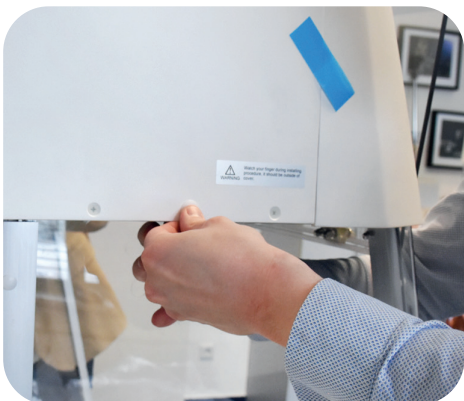
Fig. 14: Install the top housing
